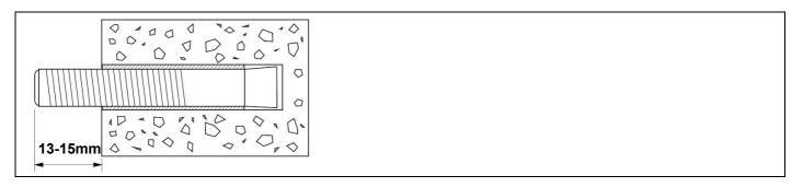
4.3 Make sure the expansion bolts are fixed securely, then mount on the air curtain and tighten the screws.
