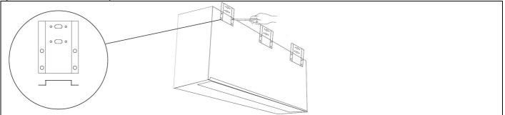
4.2 If install on concrete wall or brick wall and any other hard wall, please refer to the installation dimensions to determine the positions where fixing screws. Fix the M8 expansion bolts in the wall. Leave at least 13-15mm of the expansion bolt outside the wall.
