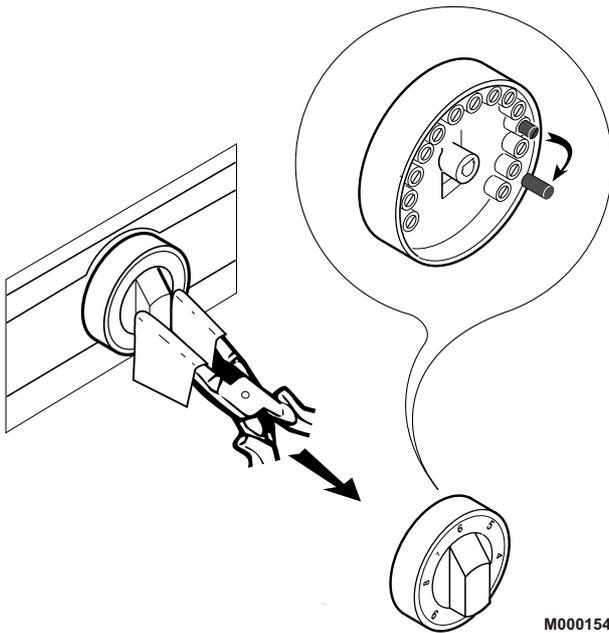
A factory-set stop limits the maximum temperature to 75 °C.
