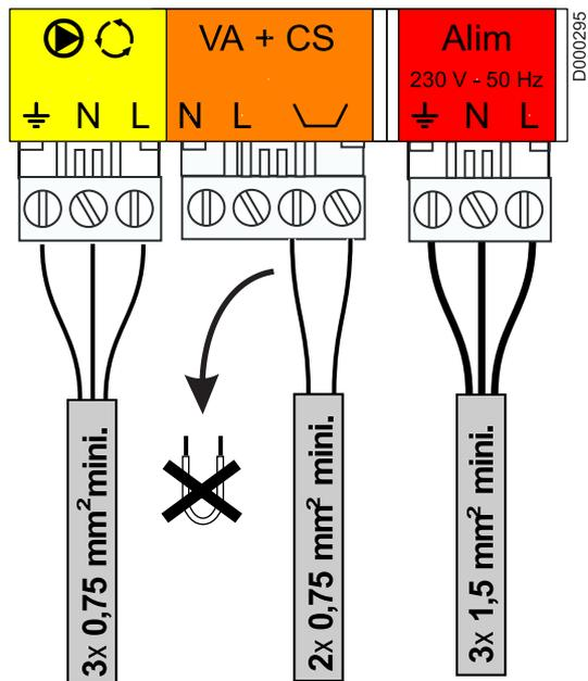
Make the electrical connection to the terminals  $\text{⏏}$ , N, L.
