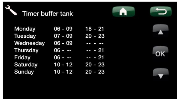
The time on the left must be lower than the time on the right for the interval to be valid.
