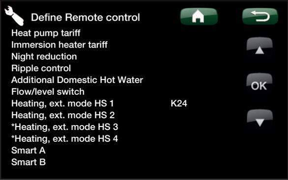
Example in which "Heating, ext. mode HS1" has been assigned terminal block "K24" for remote control.
