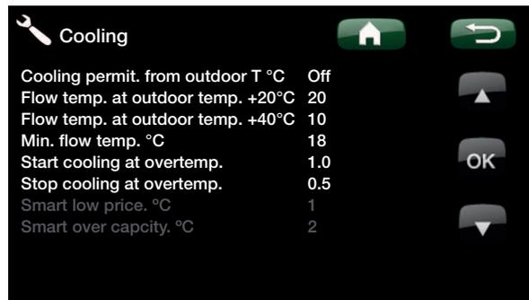
**!** The setpoint of the cooling flow is linear between +20°C and +40°C.
