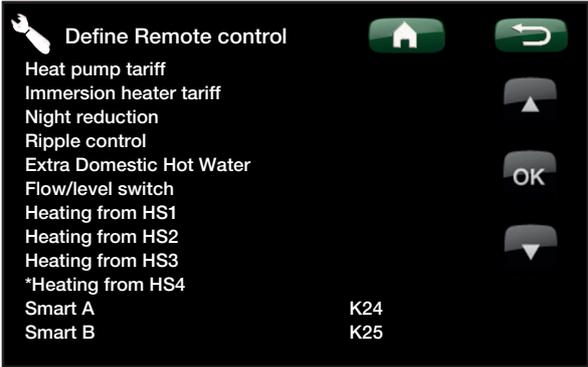
Example in which Smart A has been assigned low voltage input K24 and Smart B has been assigned low voltage input K25.
