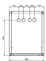
The hoses may be connected to the right, left or top or rear of the heat pump. Brine connection Ø28 mm.
