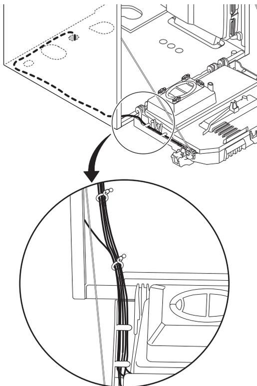
4. Connect the pump connection cable to the cable bundle by opening and closing the cable bundle bands.
