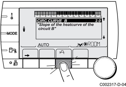
5. To modify the curve, turn the rotary button.
