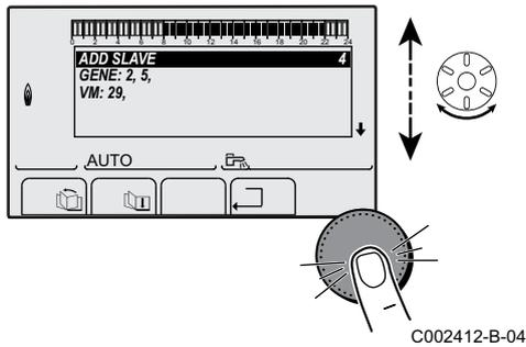
4. The screen displayed allows you to choose numbers for the slave boilers to be added to the network. Numbers 2 to 10 are dedicated to the generators and numbers 20 to 39 to the VM iSystem. Turn the rotary button to scroll through the numbers and press to confirm the number chosen. Press  to go back to the previous list.
