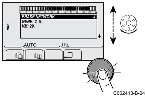
6. The screen displayed allows you to choose the numbers of the slave boilers to be removed from the network. Turn the rotary button to scroll through the numbers and press to remove the number chosen. Press  to go back to the previous list.
