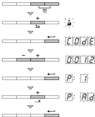
After removing a control PCB, an auto-detect must be carried out. To do this, proceed as follows:
