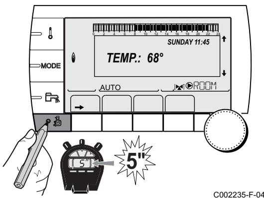
1. Access the installer level: Press key
