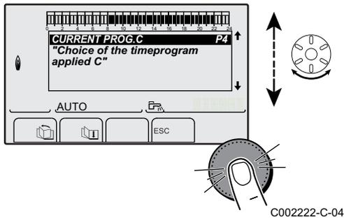
5. To modify the parameter, turn the rotary button.
