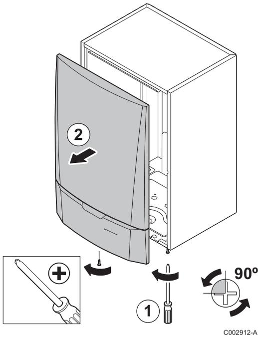
1. Unscrew the 2 screws under the front panel by a quarter turn.
