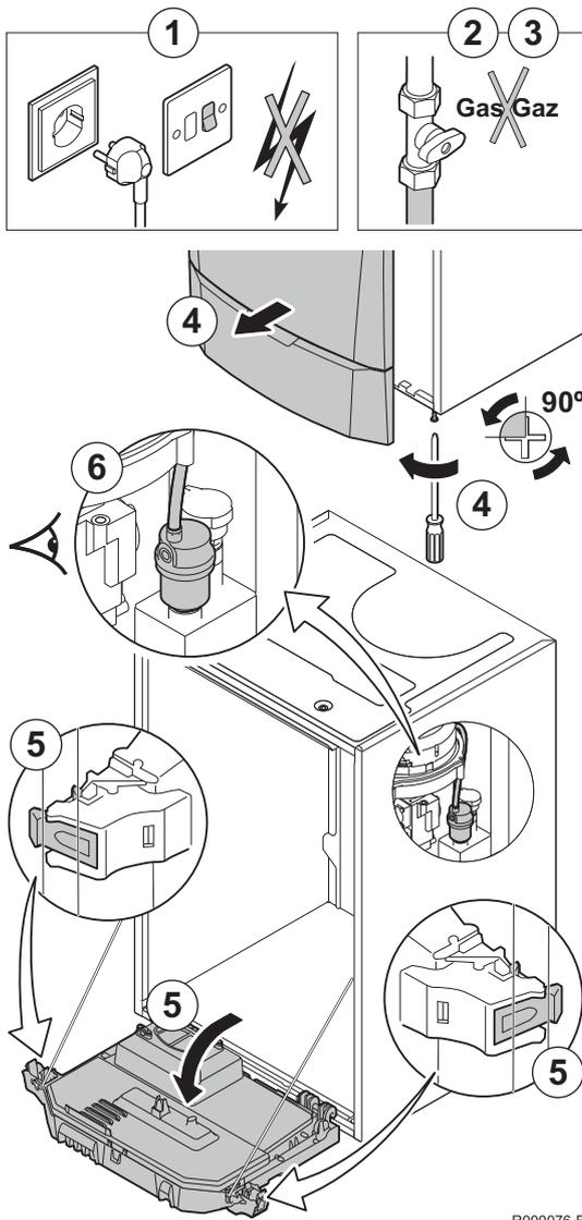
1. Switch off the boiler electrical power supply.
