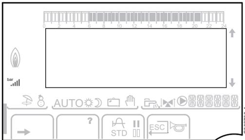
**bar** Pressure indicator: The symbol is displayed when a water pressure sensor is connected.
