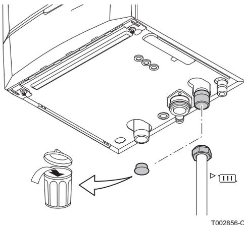
1. Remove the anti-dust plug located on the heating outlet connection (P III) under the boiler.
