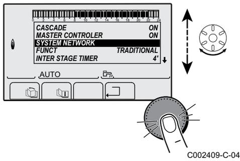
2. Select **SYSTEM NETWORK** and press the rotary button to go to the specific menu.
