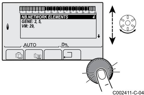
7. Select **NB. ELEMENTS.NETWORK**. This screen summarises the elements in the network recognised by the system. Press  to go back to the previous list.
